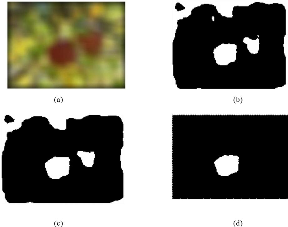
Fig. 2: Color-shape based algorithm. a) Filtered image, b) Binary image, c) Noise-reduced binary image, d) Labeled image
