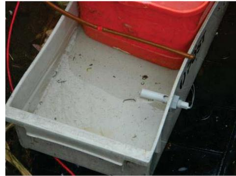
Figure 8. Evaporator for Garden Bed 2 showing the control dripper and a surface area of evaporation of 0.52 m<sup>2</sup>.
