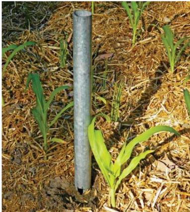
Figure 4. The steel pipe is hammered into the soil near a dripper.
