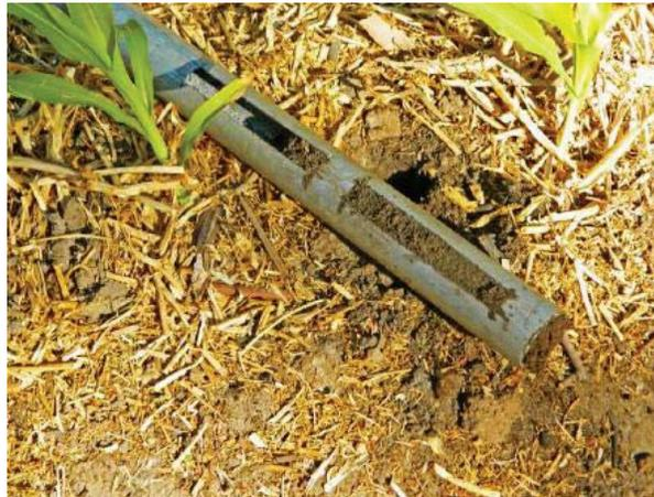
Figure 5. Check the moisture level in the core.
